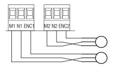
Gearmotor with encoder (M1) 24 V DC, delayed when  ${\bf closing}.$
