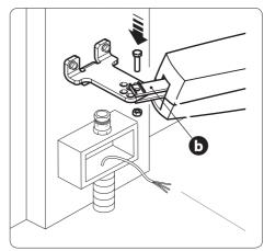
Open the gate leaf (the grub screws on the mechanical stops are loose) and fit the pin **a** into the gate bracket. Fasten using the UNI6593 washer Ø 10 and the supplied UNI 5739 M10 X 10 bolt **b a**.
